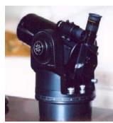
through a hole in the primary mirror to the eyepiece. The Maksutov telescope uses a thick spherical corrector lens while the Schmidt corrector plate has subtle curves. Newtonian versions of both
