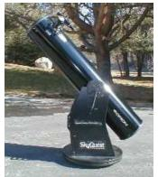
Reflectors use mirrors, coated on the front surface with aluminum, to collect and focus light. Better systems use Pyrex mirrors; cheaper telescopes have plate glass mirrors. In a Newtonian reflector
