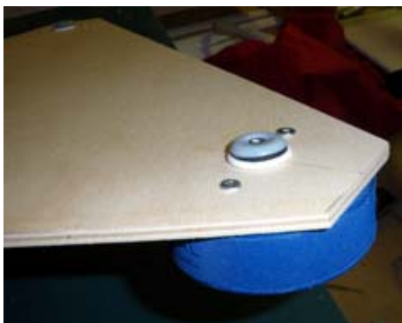
Figure 24. Pad and puck leg in position on the upper and lower sides respectively of the ground board. Note that the screw in the pad is tightened so that it is below the level of the pad surface, assuring smooth movement of the pad against the arborite on the cradle.
