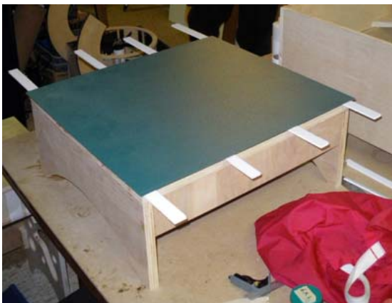
Figure 21. Technique for gluing arborite to the base of the cradle with contact cement.
