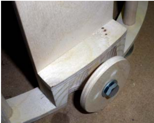
Figure 10. One of the four strut clamps on the cage. The bolt passes through the strut block and into a tee nut embedded in the vertical plate behind.
