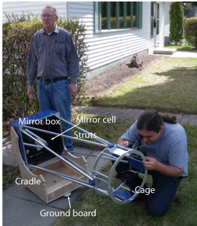
Figure 1. The completed and partially painted telescope. Victor Barbu checks the focus; "Uncle" Phil Johnson presides.
