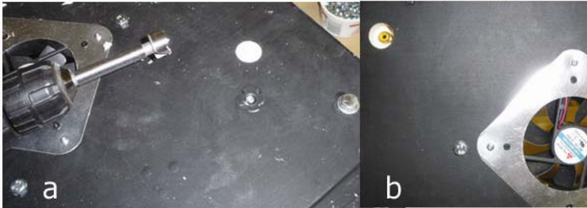
Figure 19. a) Fan in position under drill; Forstner bit and hole drilled part way through the mirror cell base board; b) Fan, with connector recessed into mirror cell base board.
