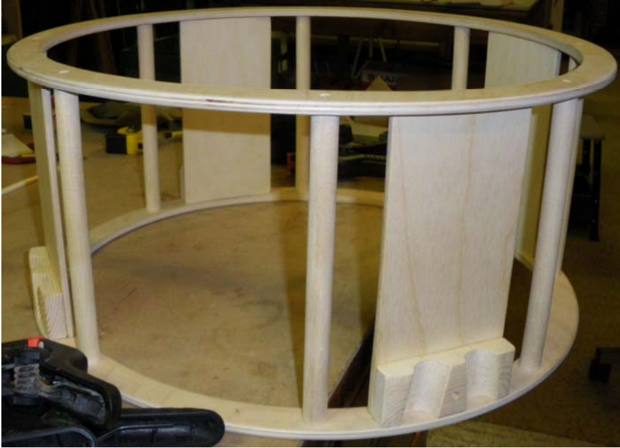
Figure 3. The cage with strut blocks and their vertical backing plates in position.
