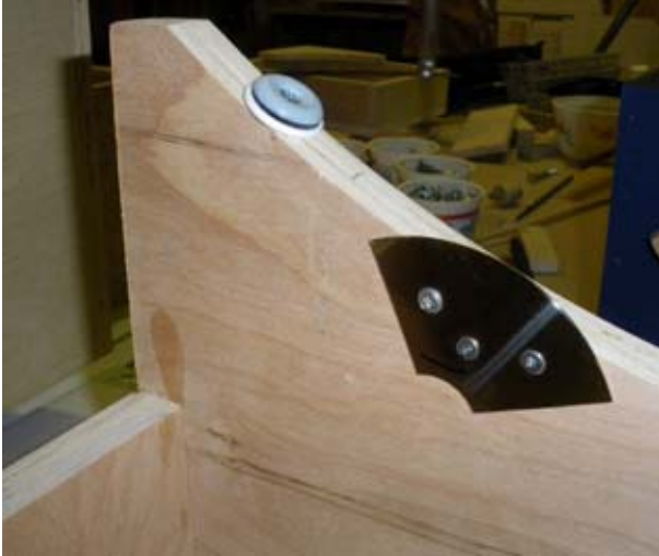
Figure 25. Part of the cradle showing placement of a glide pad and a guide.
