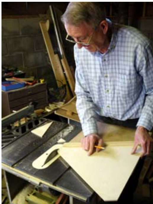
Figure 23. Phil Johnson uses a jig to cut the 60° sides and apices of the ground board.
