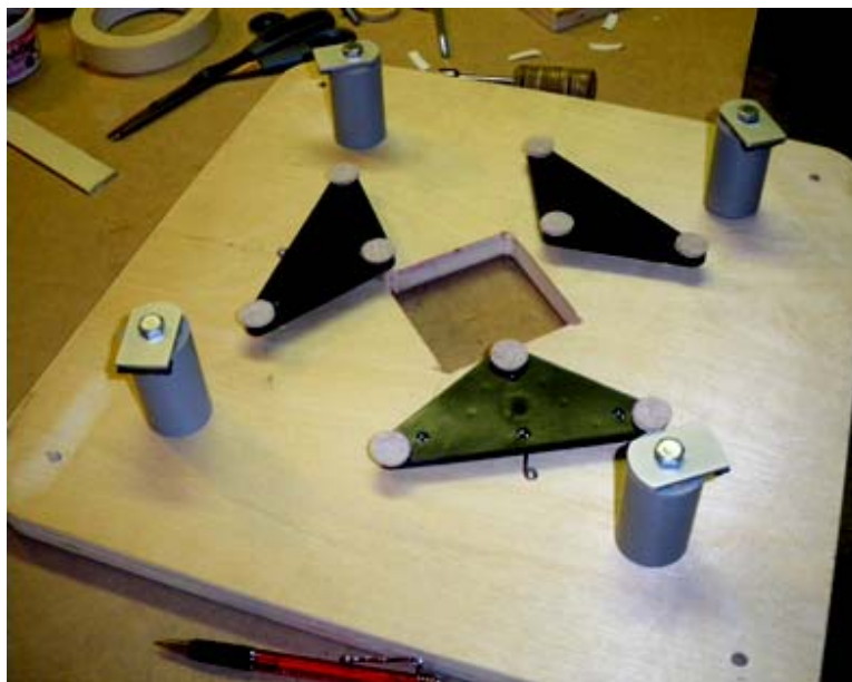
Figure 7. The mirror cell showing a central cut out for a fan, three triangular mirror supports, four mirror posts with tabs on top to prevent the mirror from tipping out of place, and a hole near each corner of the base through which bolts used in collimation will pass and attach the cell to the corner pieces in the base of the mirror box. The upper side of the cell (see 2 below) is on the left.
