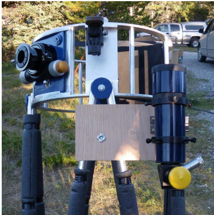
Figure 13. The revised finder system with red dot finder attached to the cage and a 9 by 60 finderscope on the finder assembly board.
