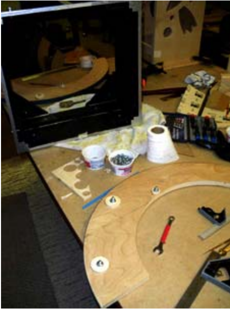
Figure 18. Side bearing spacers glued and temporarily clamped in place by bolts and nuts.
